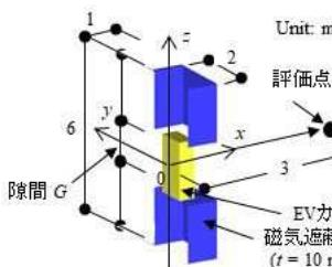
(a)磁気遮蔽材に隙間設置
