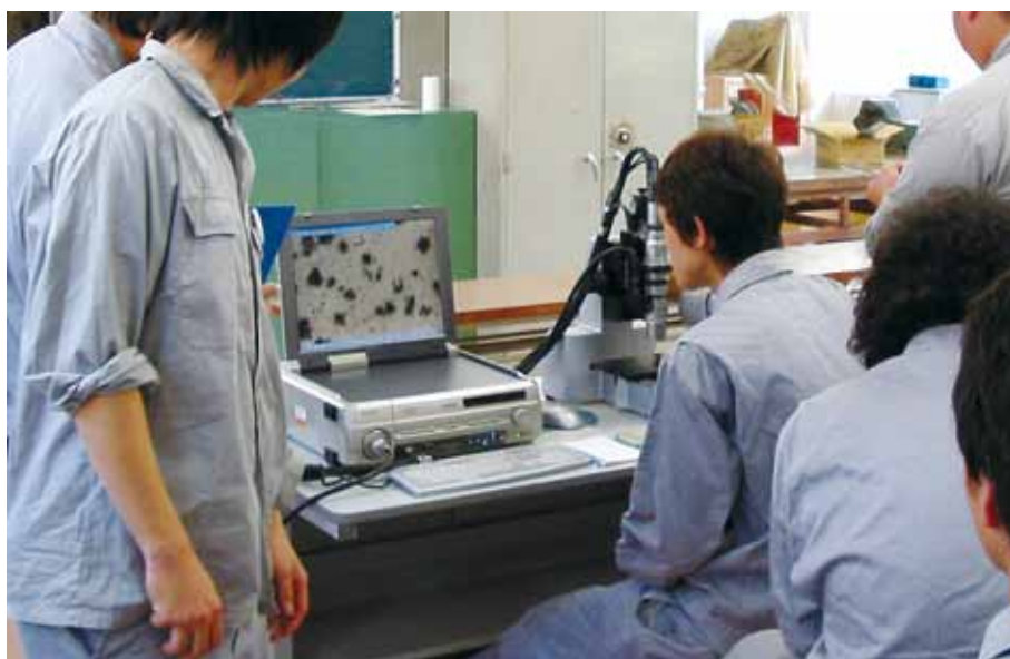
金属組織のデジタル顕微鏡観察 Observation of microstructure of metals with digital microscope
