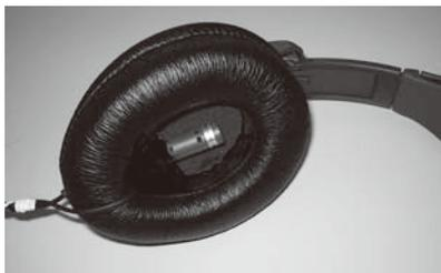
Fig.2 Headphone with Error microphone
